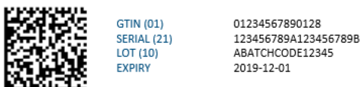
Figure 6: GTIN Coding example
